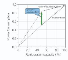
Vector frequency control is applied to reasonably distribute motor rotational torque to improve energy efficiency and save up to 38 % energy under some load conditions.
