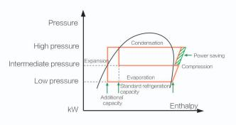
Under high compression ratio, two-stage compression makes it possible to reduce power consumption, improve system COP, and obtain lower evaporating temperature.
