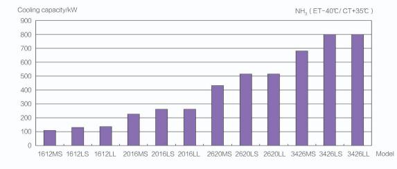
Notes: Refrigeration capacity at the rotational speed of 2,960 rpm and suction superheat of 5 °C, and with an intercooler.
